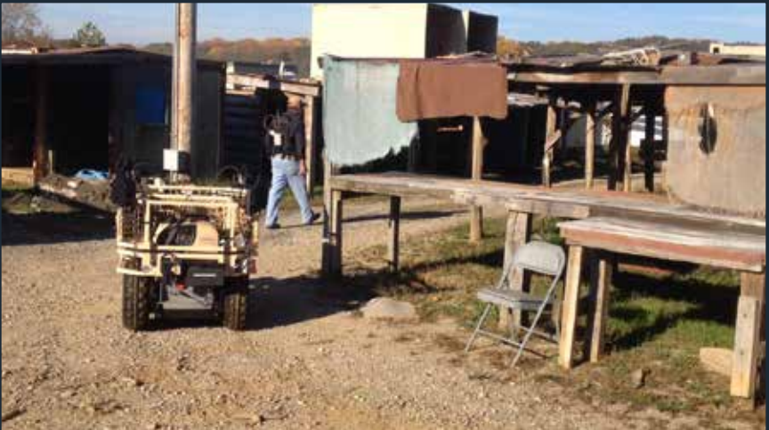
5D Robotics' Segway RMP following a human operator through a shantytown at the Intuitive Robotic Operator Control (IROC) Challenge at the Muscatatuck Urban Training Center.
